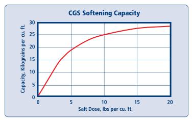
Capacity and leakage data are based on the following: 2:1 Ca:Mg ratio, 500 ppm TDS as CaCO3, 0.2% hardness in the salt and 10% brine concentration applied co-currently through the resin over 30 minutes. No engineering downgrade has been applied.
