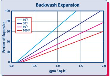
The graph above shows the expansion characteristics of ResinTech MBD-100 as a function of flow rate at various temperatures.
