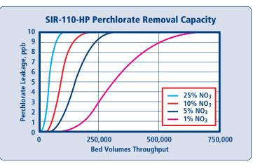
Capacity chart is based on waters with inlet conditions of 10 ppb ClO<sub>4</sub>, TDS less than 500 ppm, and is for perchlorate alone, exclusive of other anions. No engineering downgrade has been applied.
