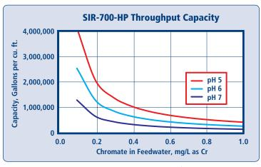
Capacity chart is based on waters with TDS less than 500 ppm and is for chromate alone, exclusive of other anions. Capacity shown is for the working bed in a worker polisher configuration. No engineering downgrade has been applied.
