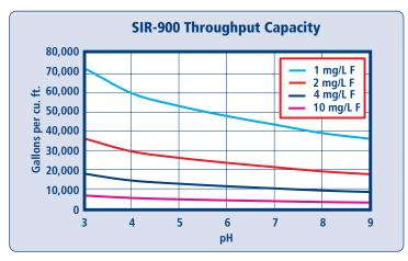
SIR-900 capacity is based on a flow rate of 1 gpm per cu. ft. and less than 500 ppm TDS as CaCO<sup>3</sup>. No engineering downgrade has been applied.
