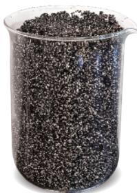
Similarly, there are virtually no packed bed residential systems and very few commercial packed bed systems operating in North America. For that reason Aldex OSM contains no floating resin. Aldex OSM uses the volume an inert plastic bead would occupy and replaces that unproductive volume with ion exchange resins able to remove hardness, tannins, iron, manganese and hydrogen sulfide.
